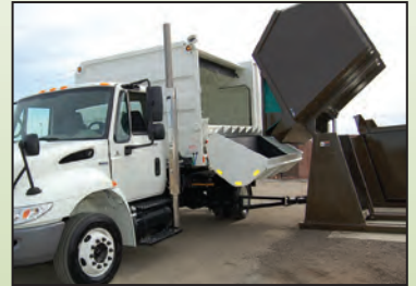
HL Arm services Hyd-A-Ways with a closed-loop hydraulic system; bucket extension packs more volume per cycle.
