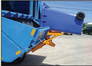
Cart tipper (shown with bucket extension) facilitates semi-automated collection of poly carts.
